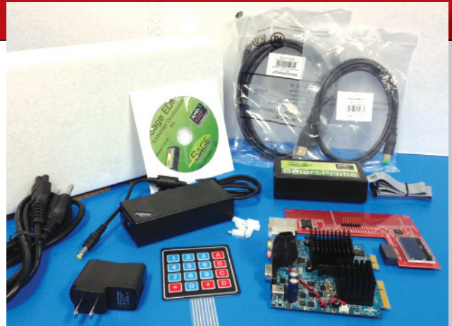
The Gizmo Explorer Kit includes the components and accessories needed to get started with embedded design.
