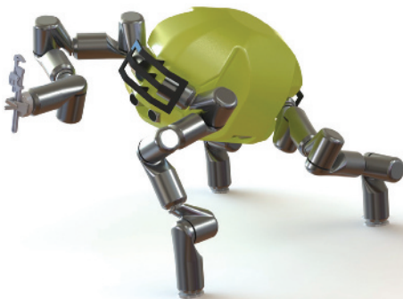
Inspired by an ape-like paradigm, RoboSimian brings human-level mobility and manipulation to disaster areas through the use of four identical limbs. Image courtesy of NASA-JPL.
